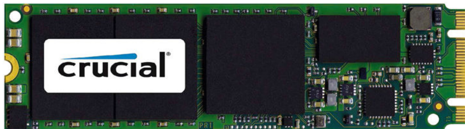
Above: Initially optimal for portable PCs, M.2 is now a common desktop storage interface.
