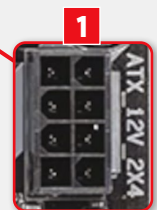
The Gigabyte H310 S2H motherboard takes power through 8-pin and 24-pin connectors
